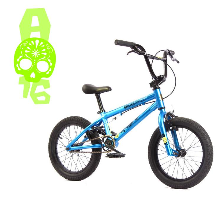
• Frame: HiTen steel, top tube length: 405mm (15.95"), RC 290mm, HT 75°
